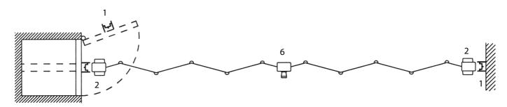
Single stack with "S" curve into pocket using 2 x 135° curves
