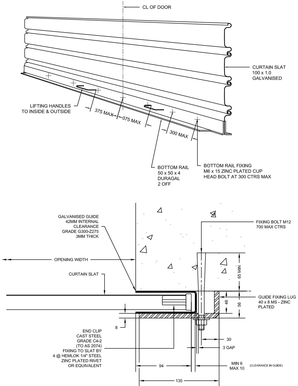
**Please Note:** This Fire Shutter is designed for use in walls and other elements of construction required to provide fire resistance. Reference should be made to the requirements of Building Code of Australia and materials tested to AS1530. This Fire Shutter should be installed in conjunction with the requirements of AS1905.2 and Exova Letter of Opinion Report #27544-07.
