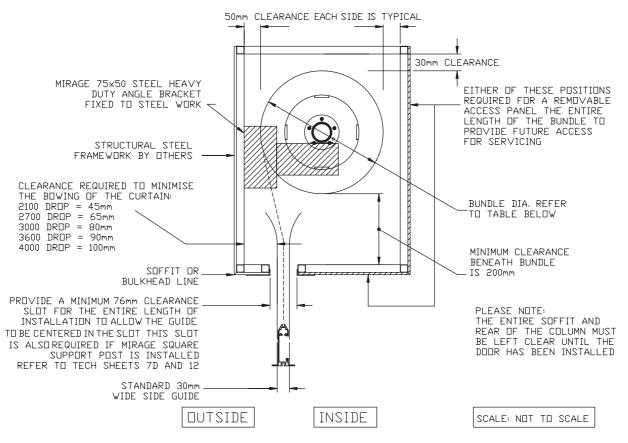
N.B THE INTERNAL END OF THE BULKHEAD MUST BE CLEAR TO AT LEAST A MINIMUM 76mm OR A RECOMMENDED 140mm FROM THE DAYLIGHT OPENING, WE THE FRONT OF THE GUIDE (REFER TO TECH SHEETS 7C AND 7D) N.B DROP HEIGHT IS MEASURED FROM SOFFIT OR BULKHEAD LINE TO THE FLOOR N.B REMOVABLE MULLIONS ARE NOT SUITABLE FOR THIS PRODUCT
