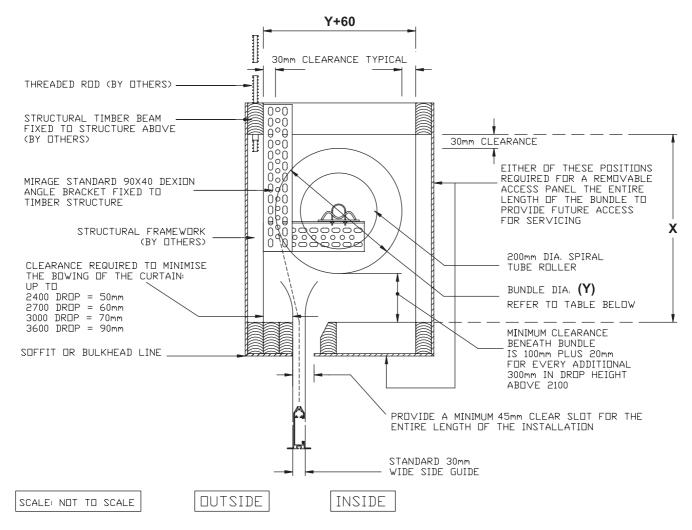
N.B THE INTERNAL END OF THE BULKHEAD MUST BE CLEAR TO AT LEAST THE BACK OF THE GUIDE OR OVERALL THE REMOVABLE SIDE MULLION
