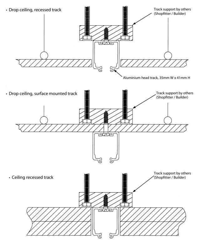
NOTE: It is unacceptable to have any gap between the track and the track support.
