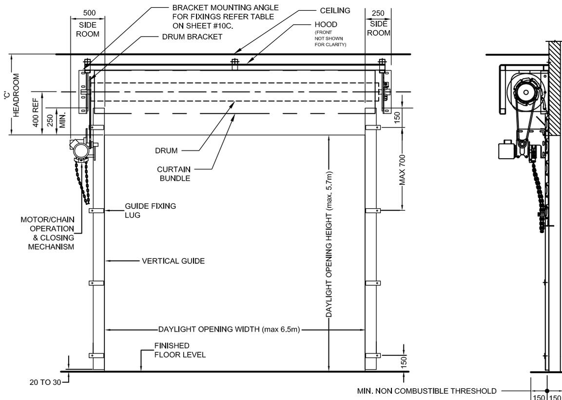
**Please Note:** This Fire Shutter is designed for use in walls and other elements of construction required to provide fire resistance. Reference should be made to the requirements of Building Code of Australia and materials tested to AS1530. This Fire Shutter should be installed in conjunction with the requirements of AS1905.2 and Exova Letter of Opinion Report #27544-07.
